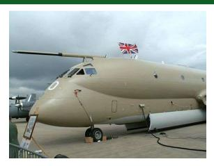
XV230 Nimrod which was lost over Afghanistan 2 September 2006, with the loss of all 14 crew on board, likely as the result of interaction between fuel and hot air systems.
